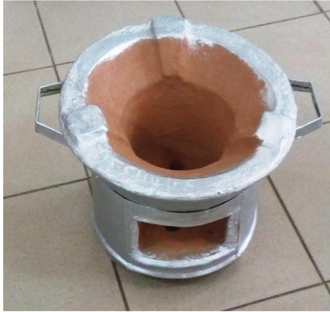
*Figure 4: The stove with metal cladding*
