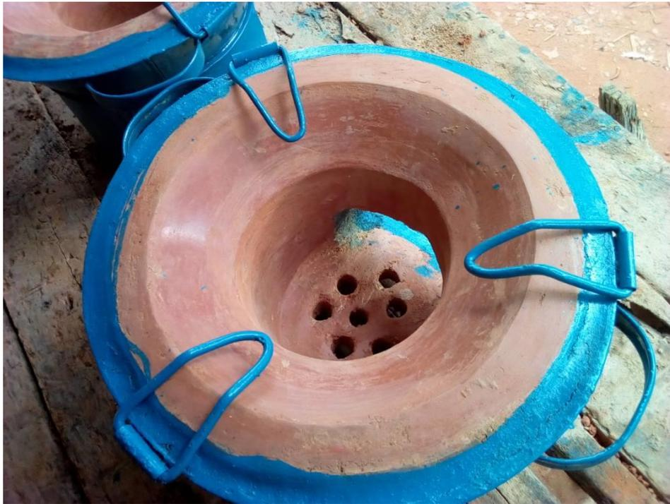
*Figure 5: Later stove model with metal pot rest*
